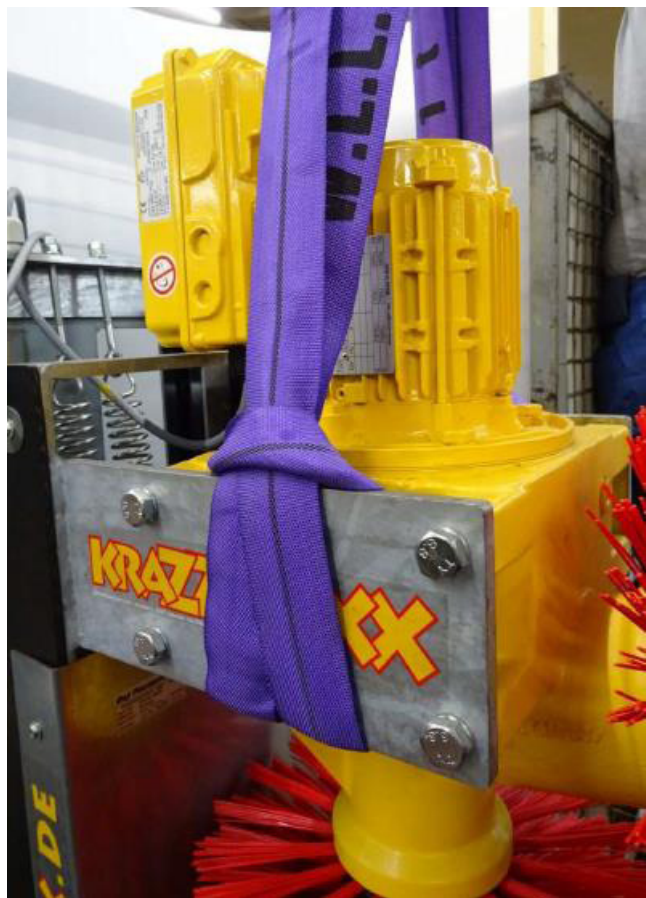
Figure 3: Affixing the lifting harness
